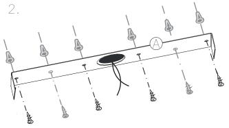
Note: When mounting be sure to locate and mount  $\bigcirc$  to a joist/celing beam
