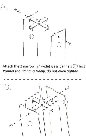
Attach the 2 wide (3" wide) glass pannels **Pannel should hang freely, do not over-tighten** Make sure the glossy side is facing outwards
