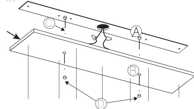
Remove rods and attach (B) to (A) with the button head screws (D)
