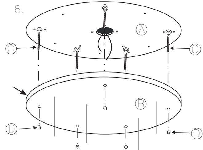
Remove rods and attach (B) to (A) with the button head screws (D)
