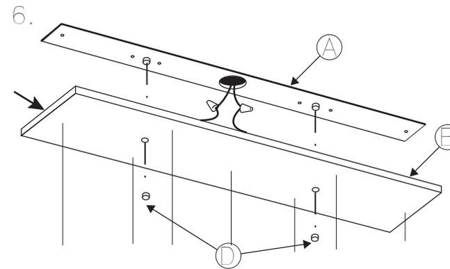
Remove rods (C) and attach (B) to (A) with the button head screws (D)
